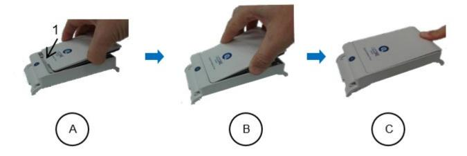
3. After all six batteries are in place, insert the protrusion at the bottom of the lid (see figure above) to its slot in the EBP, and press the latch downwards until it clicks.
